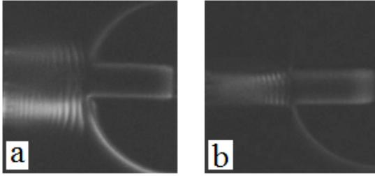
Fig. 1. (a) Open discharge [3]. (b) Limited discharge [4].
